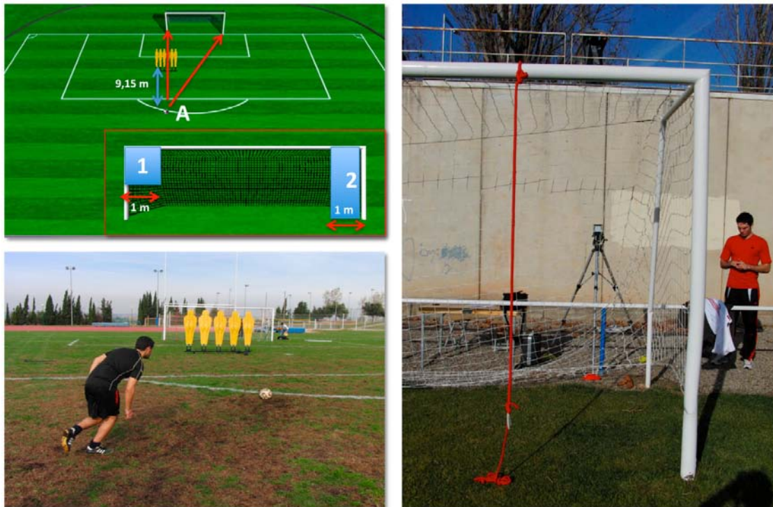
Fig. 1. Radar position (right), barrier position (left-bottom) and general protocol lengths (top-left).
