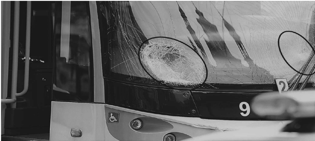
Fig. 1 Tram windscreen after a collision with two pedestrians – contact points Source: taken from [6] (photo by Michal Šula, MAFRA)
